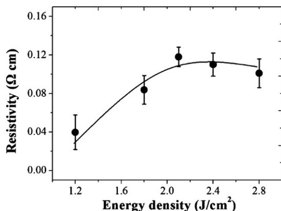
**Fig. 9.** Resistivity of ZnO films at room temperature as a function of laser energy density.
