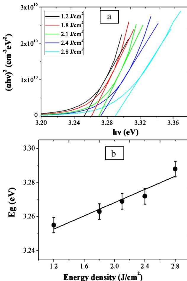
Fig. 8. (a) Plot of  $(ahv)^2$  as a function of  $(hv)$  for ZnO films deposited with different laser energy density, and (b) laser energy density dependence of the band gap energy for ZnO films.
