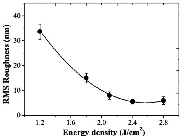
Fig. 6. The root-mean-square (RMS) surface roughness of the deposited ZnO films as a function of the laser energy density.
