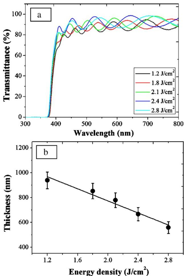
Fig. 7. (a) Transmittance spectra and (b) thickness of the deposited ZnO films as a function of the laser energy density.
