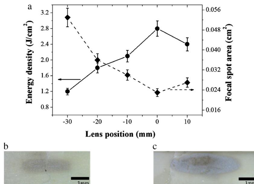
**Fig. 1.** (a) The calculated laser energy density as a function of the relative lens position. The position 0 corresponds to the lens focal distance. The measured laser spot area (single shot) is shown for (b) the highest and (c) the lowest energy density.
