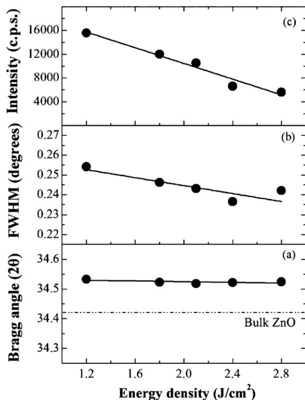
Fig. 3. (a) Bragg angle of the (002) diffraction peak, (b) FWHM and (c) intensity as a function of laser energy density.
