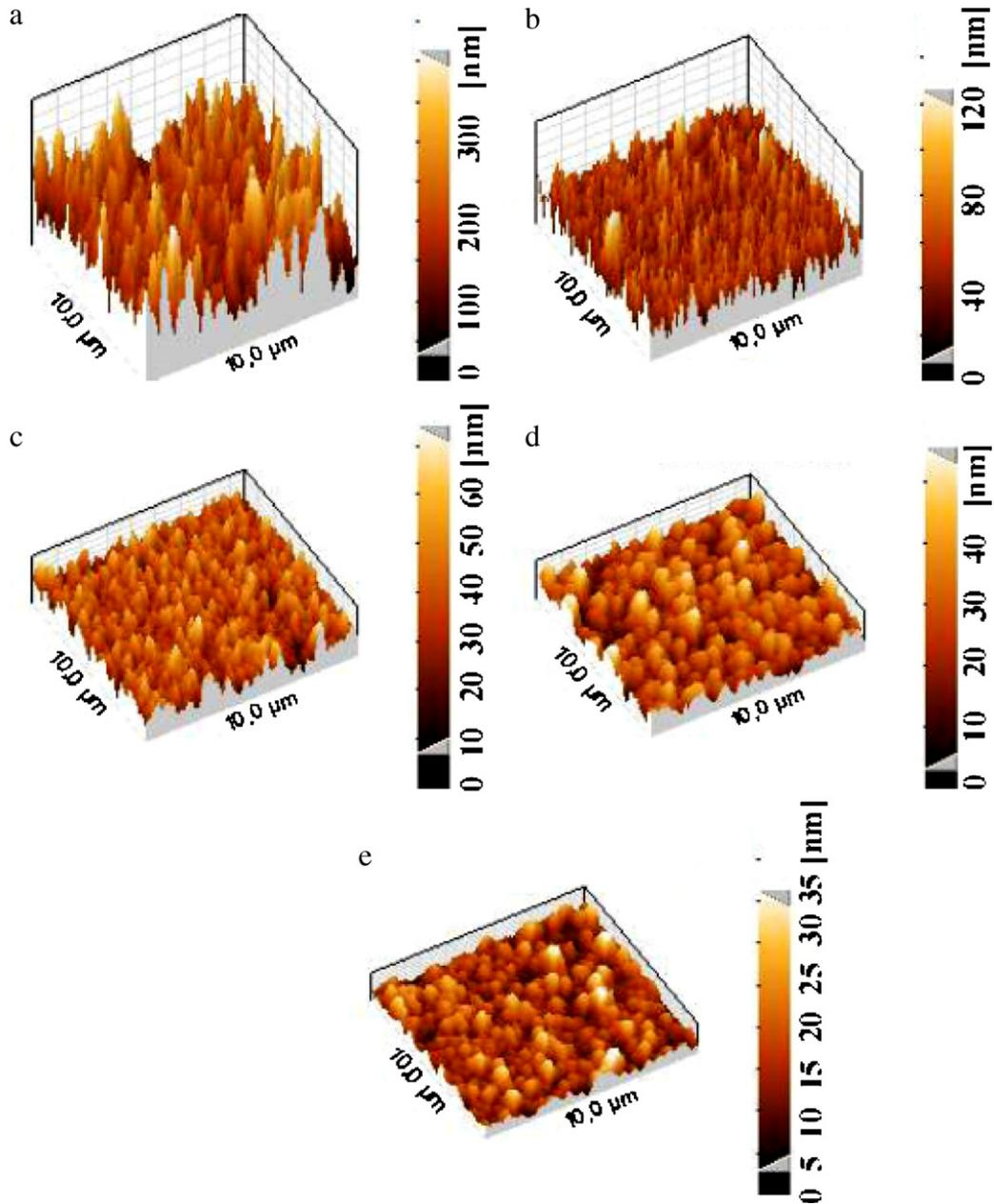
Fig. 5. AFM images of the ZnO films deposited at different laser energy densities: (a) 1.2 J/cm<sup>2</sup>, (b) 1.8 J/cm<sup>2</sup>, (c) 2.1 J/cm<sup>2</sup>, (d) 2.4 J/cm<sup>2</sup>, (e) 2.8 J/cm<sup>2</sup>.
