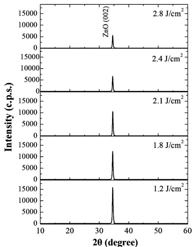
**Fig. 2.** X-ray diffraction pattern of ZnO thin films deposited at various laser energy densities.
