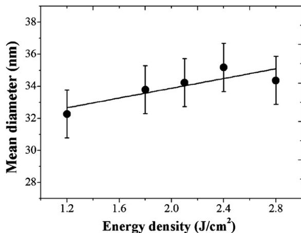
Fig. 4. The mean grain diameter of the ZnO films grown at different laser energy densities.
