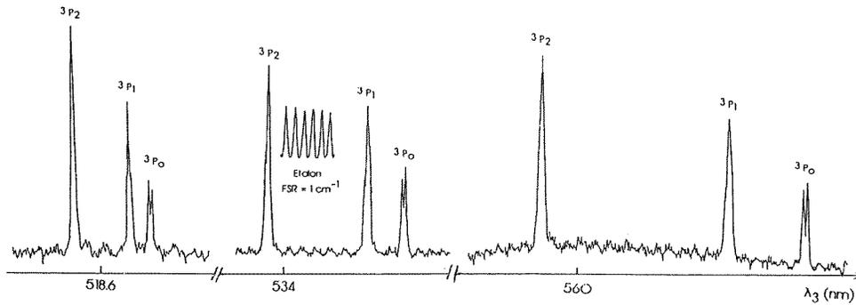
**Figure 3.** The three-step excitation spectrum  $5snp$  for  $n = 9-11$  (from right to left), recorded with the excitation scheme (b). The doublet in the  $J = 0$  component is due to the HFS splitting of the  $5s6s\ ^3S_1$  intermediate state.
