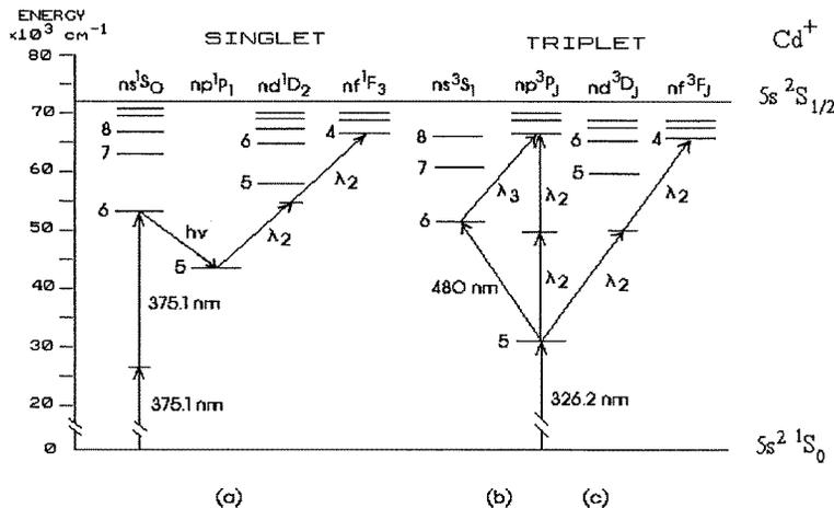
**Figure 2.** Part of the Cd energy level diagram with the various laser excitation schemes used in this experiment.
