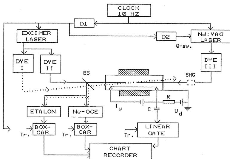
**Figure 1.** Experimental set-up: D1, D2 delays; Q-sw, Q switching of the Nd:YAG laser; BS, beam splitter; Tr, trigger pulses; SHG, second harmonic generating crystal;  $U_d$ , diode voltage;  $I_w$ , wire heating current;  $R$ , resistor;  $C$ , coupling capacitor; OGE, neon optogalvanic spectrum.
